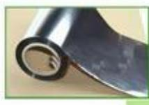
Aluminum foil is a kind of hot stamping material which directly presses a aluminum metal into leaflike film. Its hot stamping effect is similar with the pure silver foil. So it is also called false silver foil.
