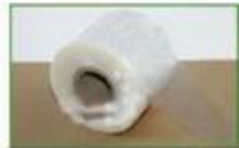
PE, short for polyethylene, is a kind of thermoplastic resin, polymerized from ethylene.
