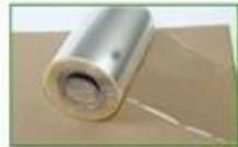
BOPP is short for "Biaxially Oriented Polypropylene", meaning two-way tensile Polypropylene film.
